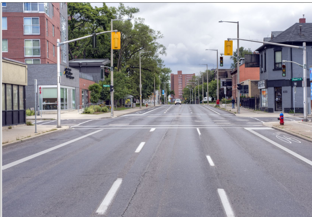
Figure 111 — Image: One-Way Street with Contraflow Bicycle Lane
