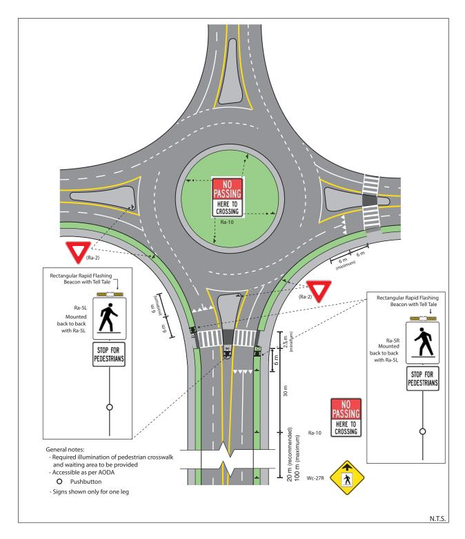
Figure 38: Pedestrian Crossover Level 2 Type C – Double-Lane Roundabout
