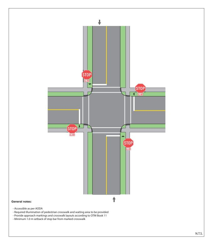
Figure 48: Stop Controlled Intersections as Pedestrian Crossing Treatment
