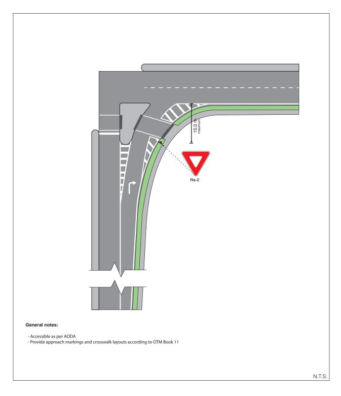
Figure 49: Yield Controlled Intersections as Pedestrian Crossing Treatment
