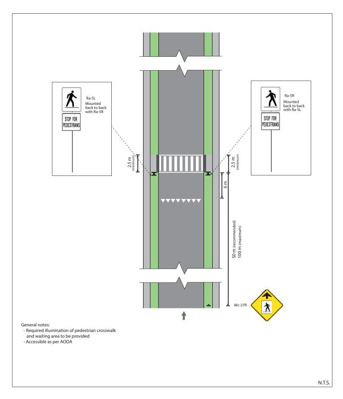
Figure 41: Pedestrian Crossover Level 2 Type D – Mid-block (1-lane, 1-way)
