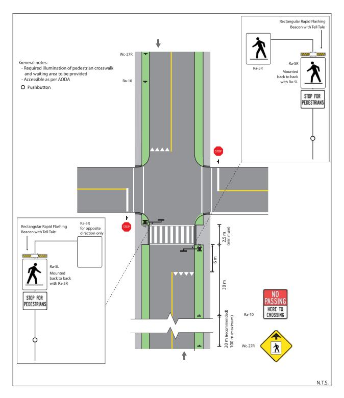
Figure 27: Pedestrian Crossover Level 2 Type B – Intersection (2-way)
