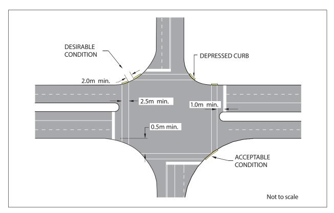
Figure 7: Typical Crosswalk Design with Standard Crosswalk Markings
