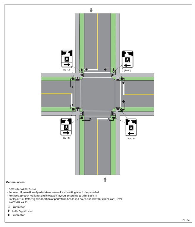
Figure 13: Pedestrian Treatment at Full Traffic Signal (2-lane, 2-way)
