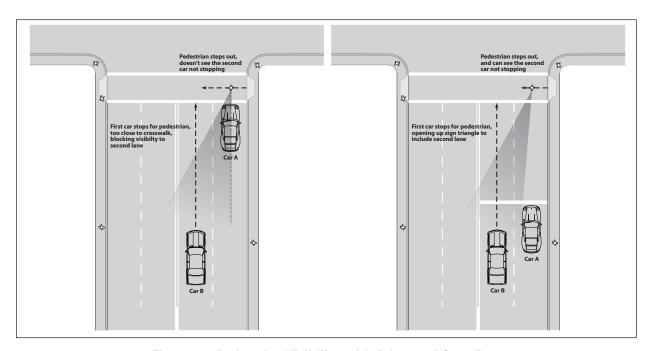
Figure 10: Pedestrian Visibility with Advanced Stop Bar
