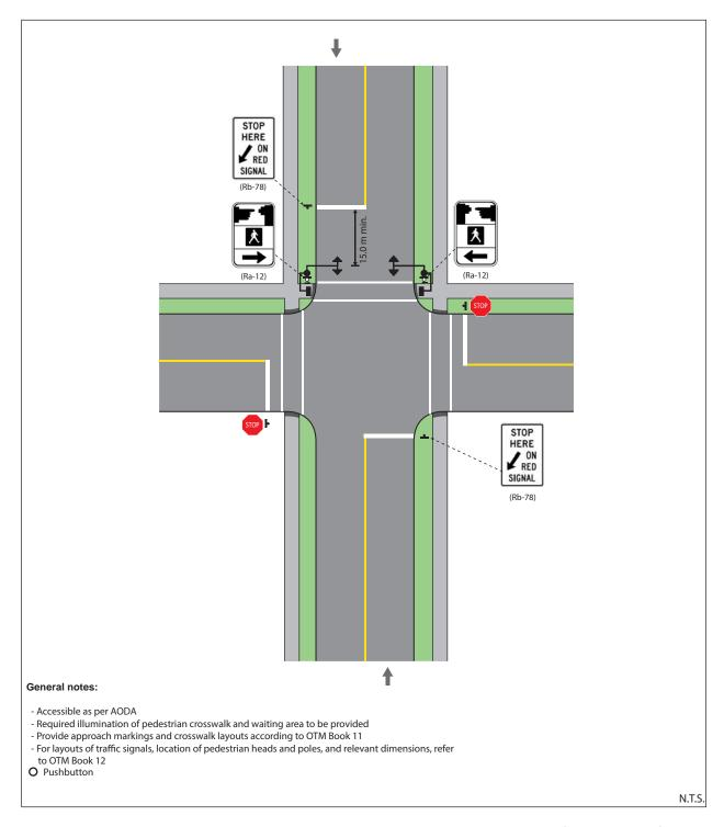
Figure 15: Intersection Pedestrian Signal Pedestrian Crossing Treatment (2-lane, 2-way)
