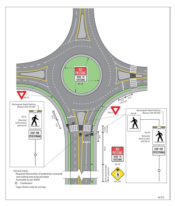
Figure 29: Pedestrian Crossover Level 2 Type B – Double-Lane Roundabout
