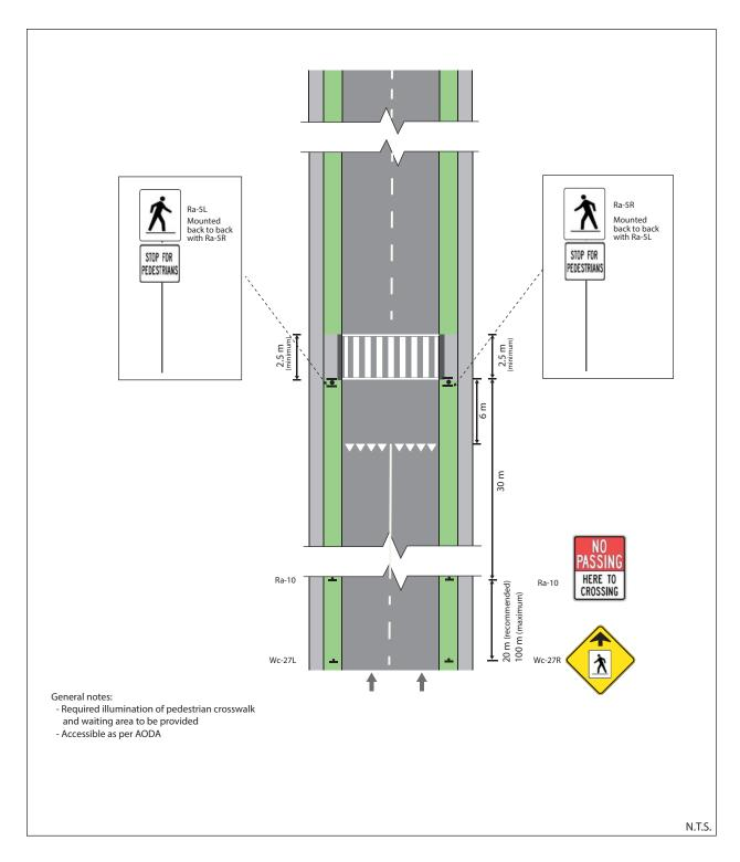
Figure 42: Pedestrian Crossover Level 2 Type D – Mid-block (2-lane, 1-way)
