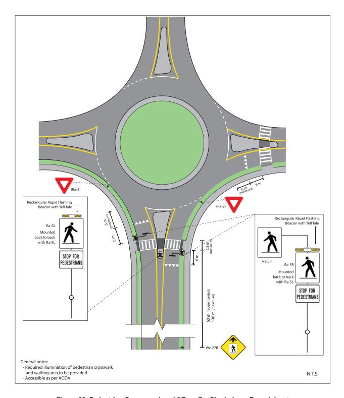
Figure 28: Pedestrian Crossover Level 2 Type B – Single-Lane Roundabout
