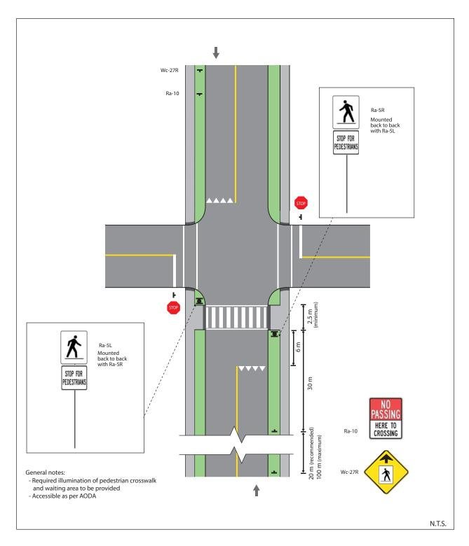
Figure 44: Pedestrian Crossover Level 2 Type D – Intersection (2-way)
