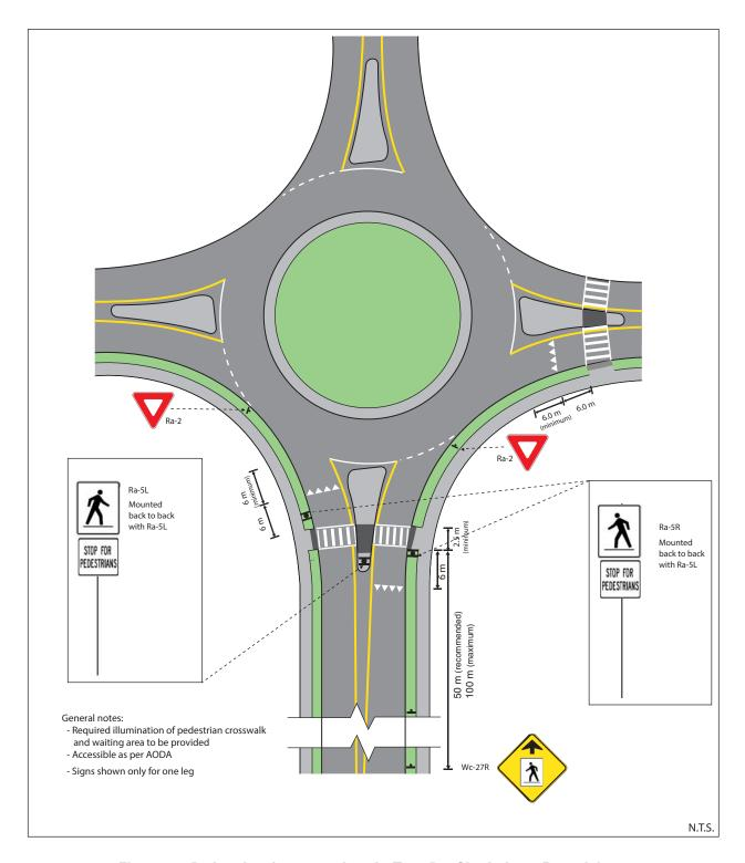
Figure 45: Pedestrian Crossover Level 2 Type D – Single-Lane Roundabout
