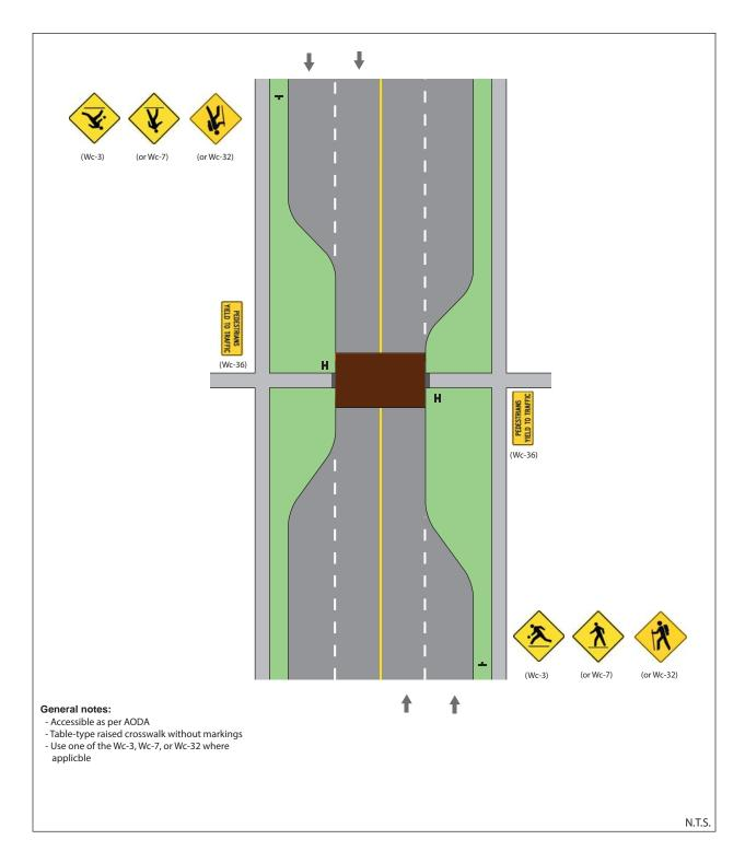
Figure 53: Typical Uncontrolled Pedestrian Crossing with Raised Crosswalk
