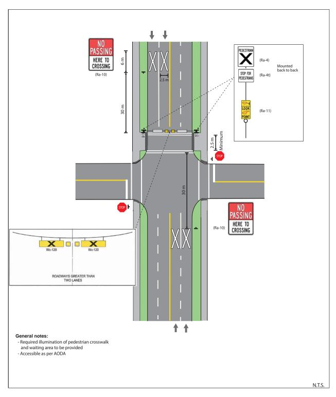
Figure 19: Pedestrian Crossover Level 1 Type A – Intersection (2-way)
