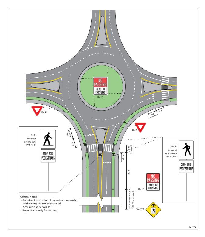
Figure 46: Pedestrian Crossover Level 2 Type D – Double-Lane Roundabout
