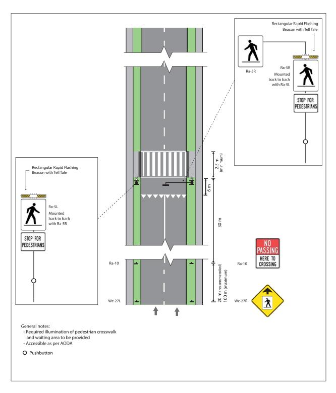
Figure 25: Pedestrian Crossover Level 2 Type B – Mid-block (2-lane, 1-way)
