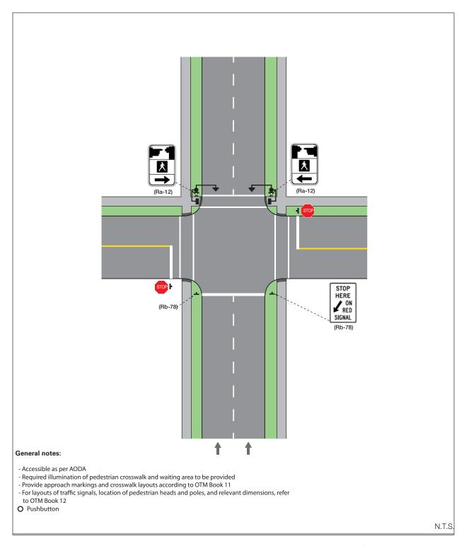
Figure 16: Intersection Pedestrian Signal Pedestrian Crossing Treatment (2-lane, 1-way)
