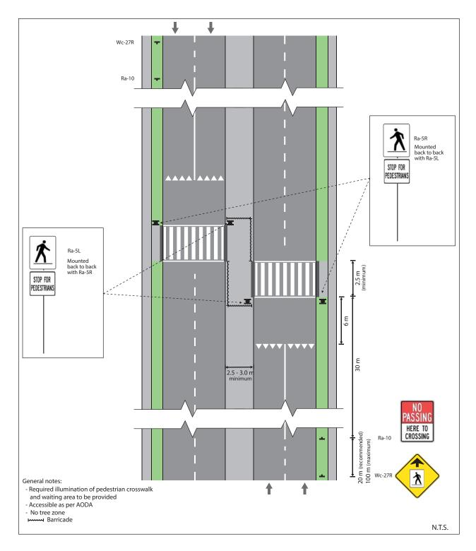
Figure 40: Pedestrian Crossover Level 2 Type D – Mid-block (4-lane, 2-way with raised refuge)
