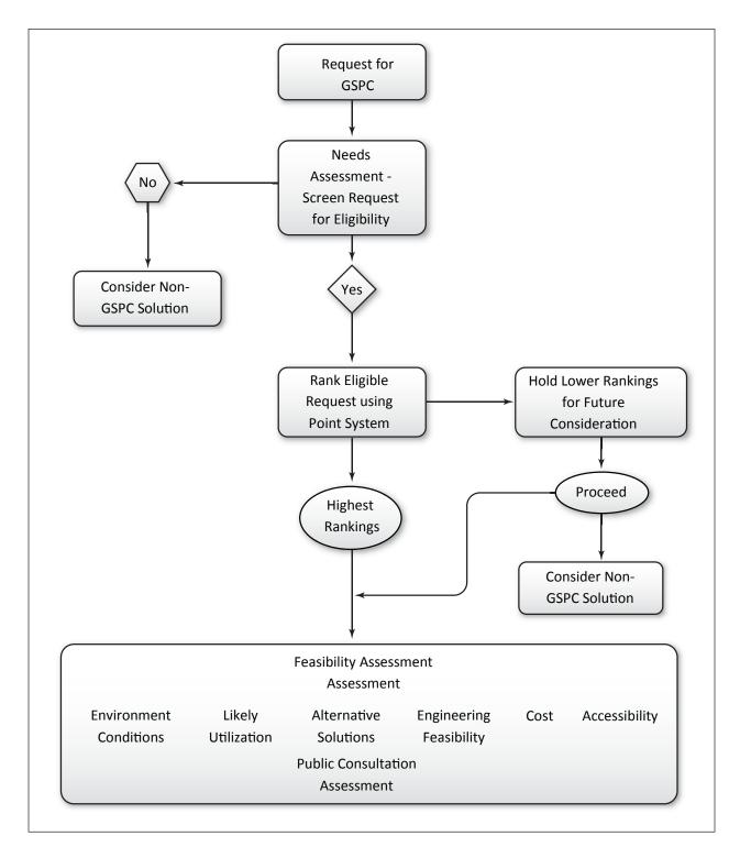
Figure 54: Grade Separated Pedestrian Crossing Feasibility Study Process
