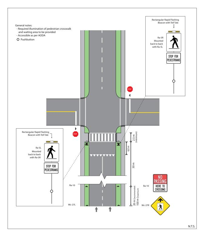
Figure 35: Pedestrian Crossover Level 2 Type C – Intersection (1-way)
