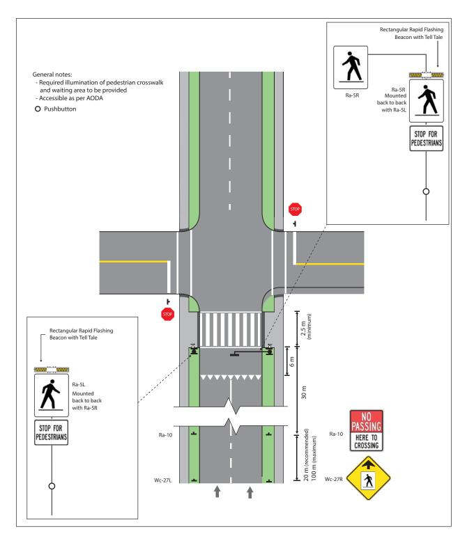
Figure 26: Pedestrian Crossover Level 2 Type B - Intersection (1 -way)
