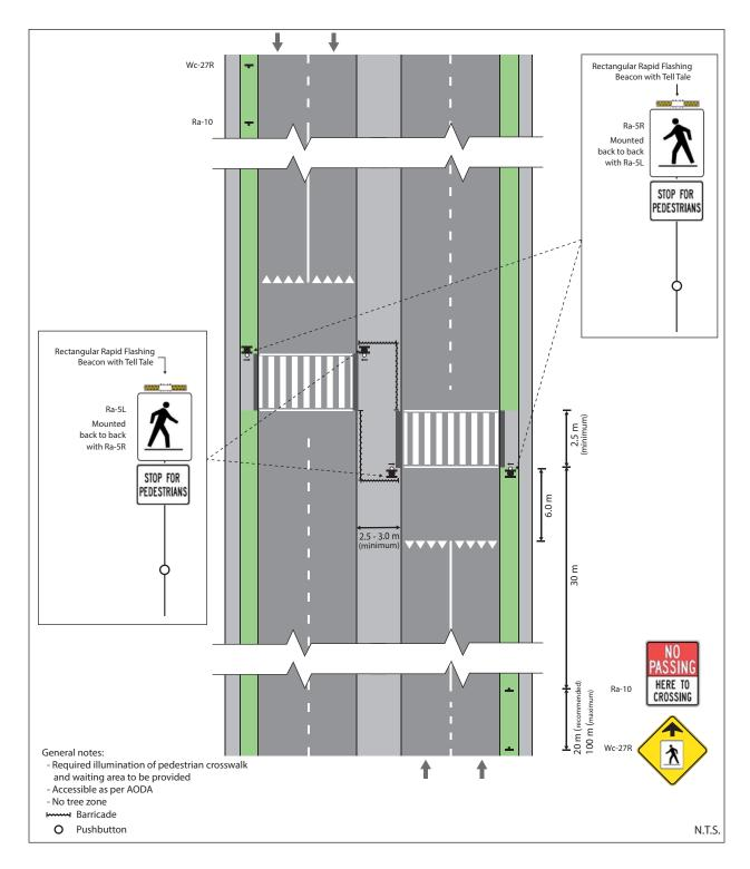
Figure 32: Pedestrian Crossover Level 2 Type C – Mid-block (4-lane, 2-way with raised refuge)
