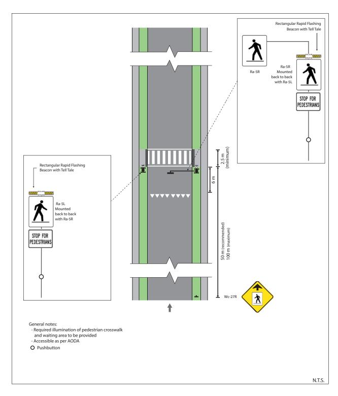
Figure 24: Pedestrian Crossover Level 2 Type B – Mid-block (1-lane, 1-way)
