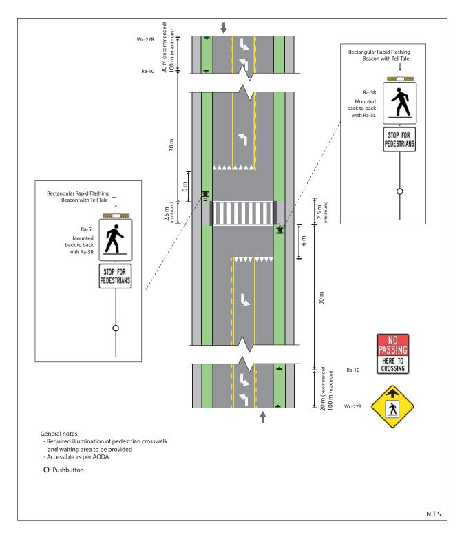
Figure 31: Pedestrian Crossover Level 2 Type C – Mid-block (3-lane with centre 2-way left-turn lane)
