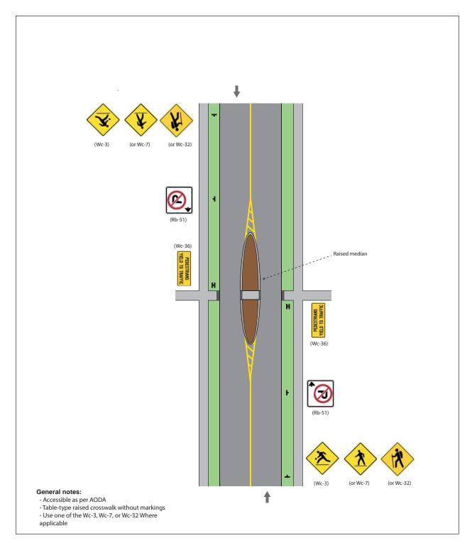
Figure 52: Typical Uncontrolled Pedestrian Crossing with Raised Median
