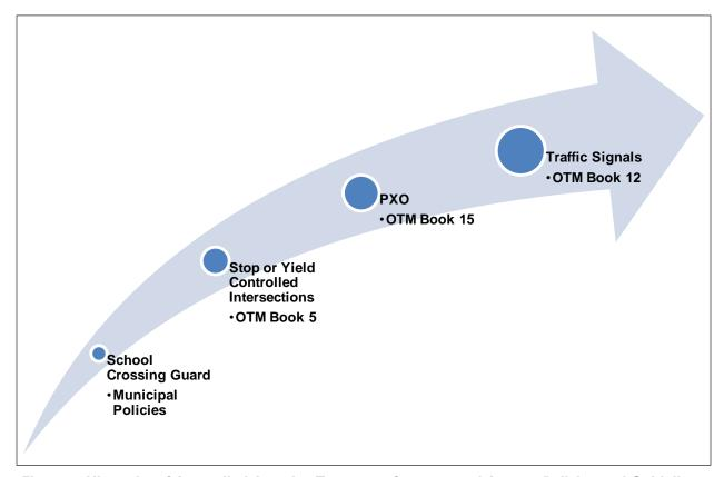
Figure 1: Hierarchy of Controlled Crossing Treatment Systems and Current Policies and Guidelines
