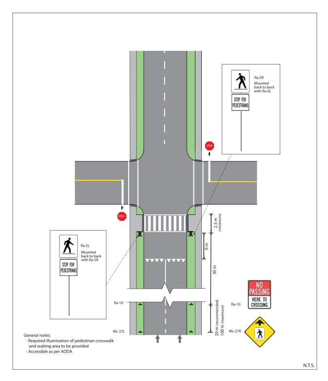
Figure 43: Pedestrian Crossover Level 2 Type D - Intersection (1-way)
