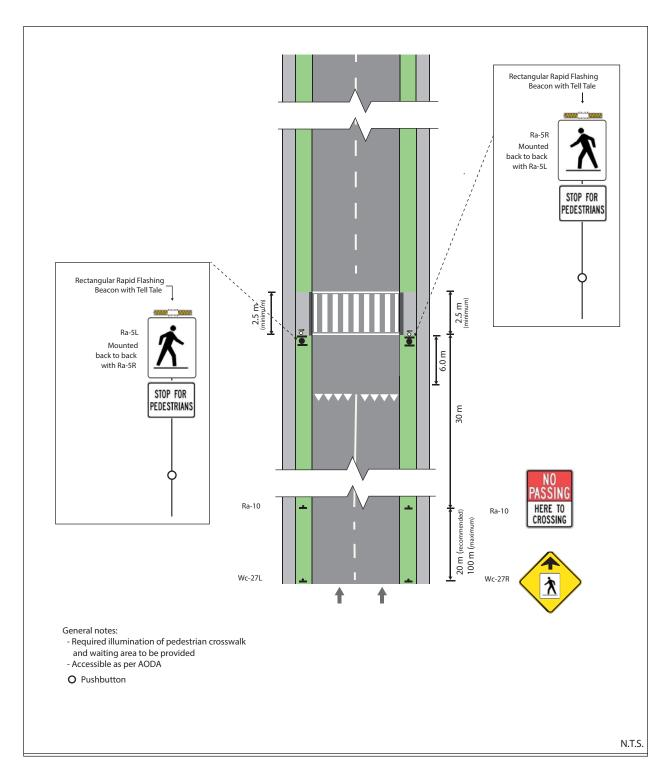
Figure 34: Pedestrian Crossover Level 2 Type C - Mid-block (2-lane, 1-way)
