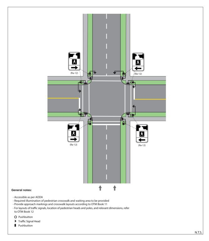
Figure 14: Pedestrian Treatment at Full Traffic Signal (2-lane, 1-way)
