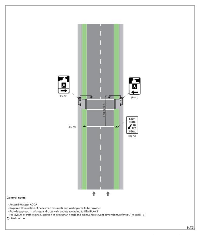
Figure 18: Mid-block Pedestrian Signal Pedestrian Crossing Treatment (2-lane, 1-way)
