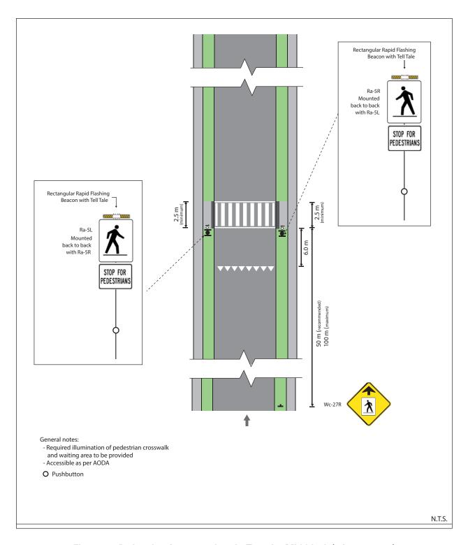
Figure 33: Pedestrian Crossover Level 2 Type C – Mid-block (1-lane, 1-way)
