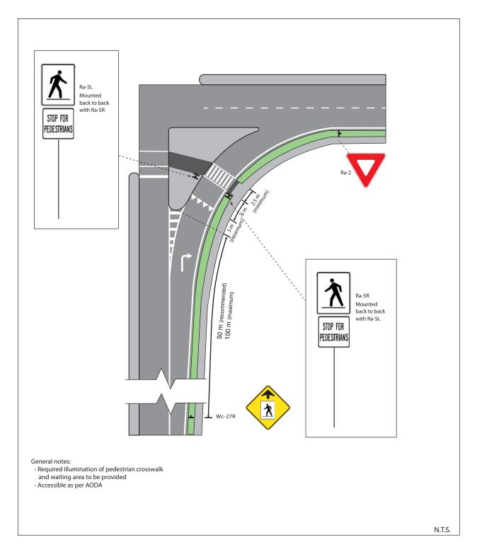
Figure 47: Pedestrian Crossover Level 2 Type D – Right-turn Channel
