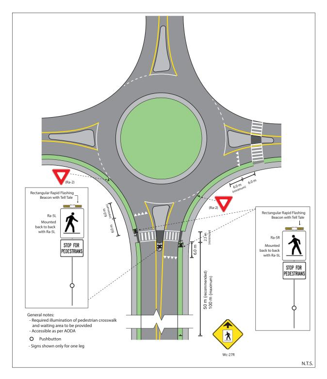
Figure 37: Pedestrian Crossover Level 2 Type C – Single-Lane Roundabout
